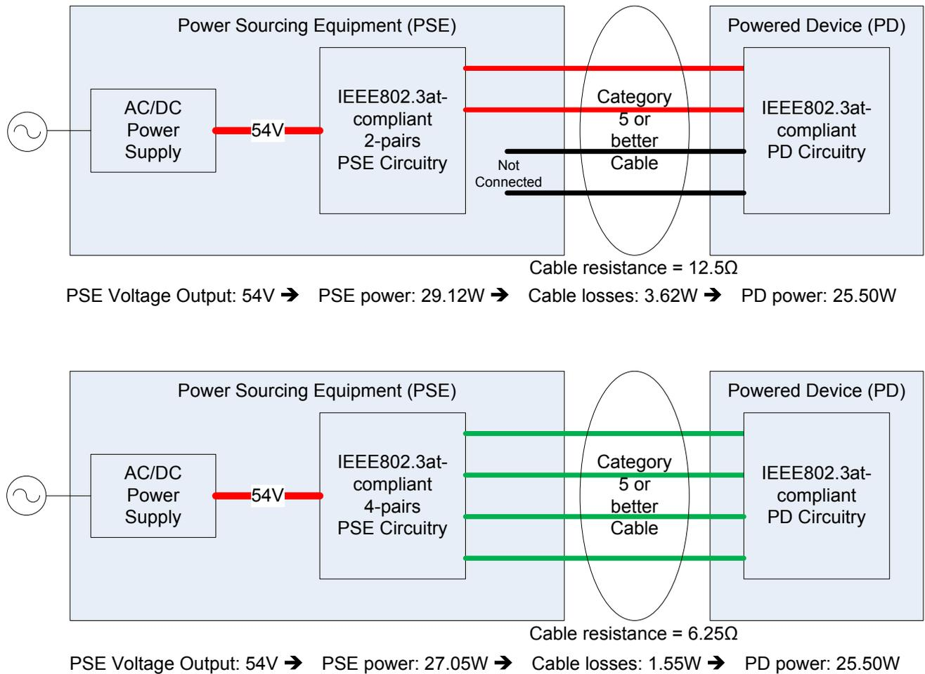
Figure 1: PoE vs. EPPoE Cable losses when powering a 25.50W PD from 54V PSE power supply
