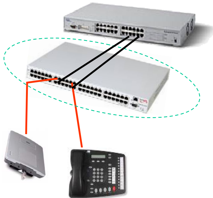
Figure 2: Midspan PoE Deployment
