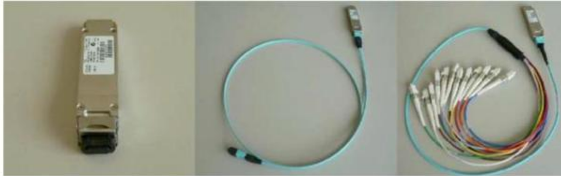
40GBASE-SR4 QSFP+ Module and Fiber Cables
