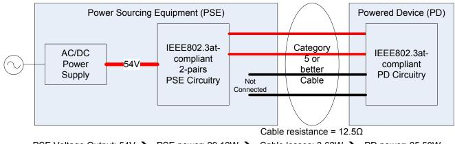
PSE Voltage Output: 54V → PSE power: 29.12W → Cable losses: 3.62W → PD power: 25.50W
