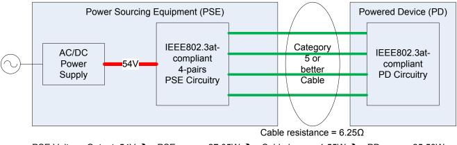
PSE Voltage Output: 54V → PSE power: 27.05W → Cable losses: 1.55W → PD power: 25.50W
